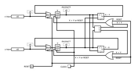
6. A version of the GCD circuit that uses this approach is shown below:
